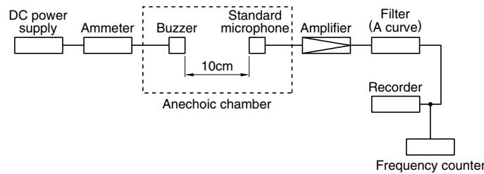
• 20dB is subtracted from the 10cm measured value, and converted to 1m value.
