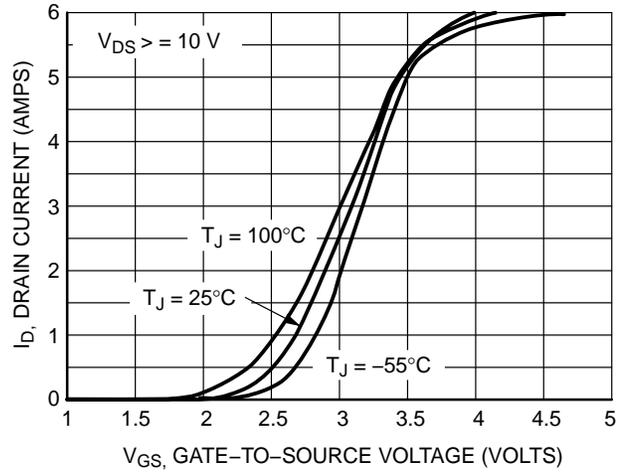
**Figure 2. Transfer Characteristics**
