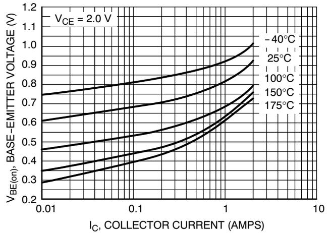
Figure 5. Base-Emitter Voltage
