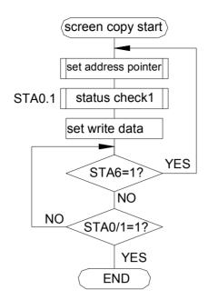
This command is available when hardware column number and software column number are the same. Hardware column number is related to MD2 and MD3 setting. Software column number is related to set text area and set graphic area command.
