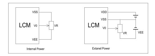
$V_0 \sim V_{SS}$ : LCD Driving voltage
