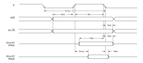
Note: tcyc6 indicates the interval during which CS is LOW and E is HIGH.
