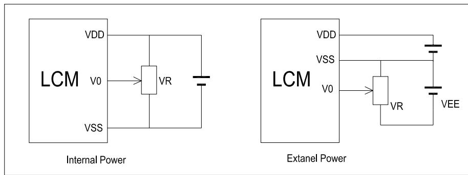
$V_{DD}-V_0$ : LCD Driving voltage
