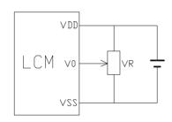
VDD~V0: LCD Driving voltage
