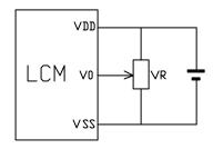
VDD~V0: LCD Driving voltage
