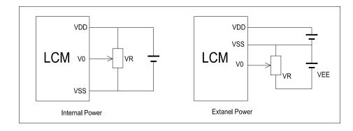
$V_{DD^{\sim}}V_0\text{: LCD Driving voltage}$
