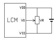
VDD~V0: LCD Driving voltage
