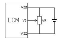
$V_{DD\sim}V_0$ : LCD Driving voltage
