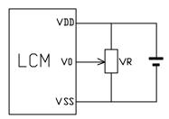
VDD~V0: LCD Driving voltage VR: 10k~20k
