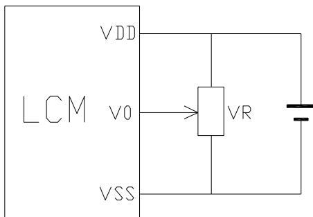
V<sub>DD</sub>-V<sub>0</sub>: LCD Driving voltage
