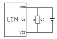
VDD~V0: LCD Driving voltage
