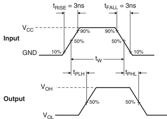
**Figure 3. AC Waveforms**
