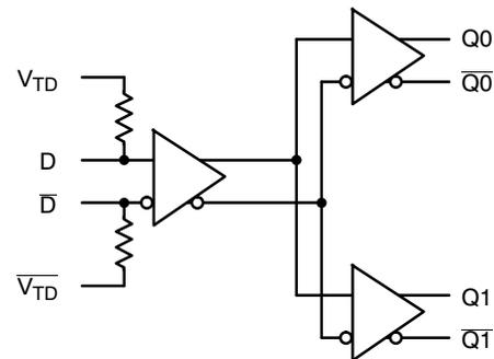
Figure 1. Logic Diagram
