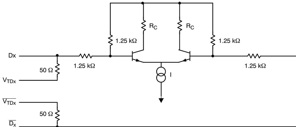
**Figure 6. Input Structure**
