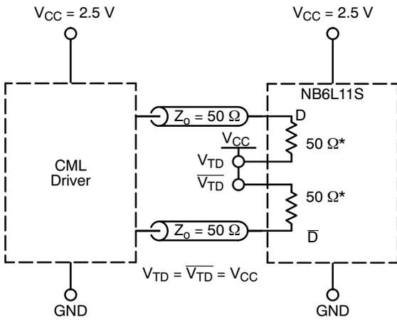
Figure 9. Standard 50  $\Omega$  Load CML Interface
