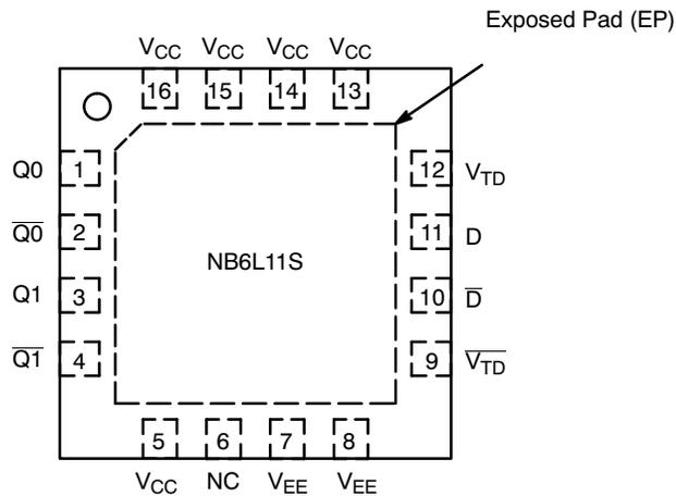
Figure 3. NB6L11S Pinout, 16-pin QFN (Top View)
