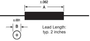
Leads smaller than 0.020 are Grade A Nickel. Leads of 0.020 diameter and larger are tinned copper. Other lead materials and diameters are available, please call the factory.
