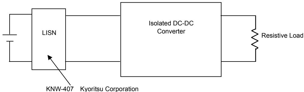
(Note) Measurement at Radiation Noise, Conductive Noise, Output ripple & Noise.
