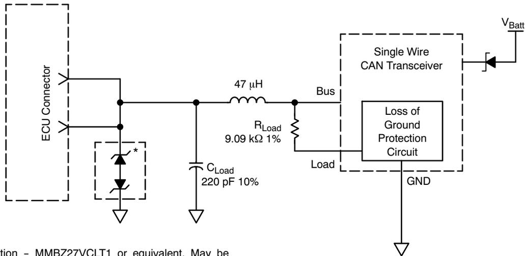
\*ESD Protection - MMBZ27VCLT1 or equivalent. May be located in each ECU ( $C_{Load}$  needs to be reduced accordingly) or at a central point near the DLC.
