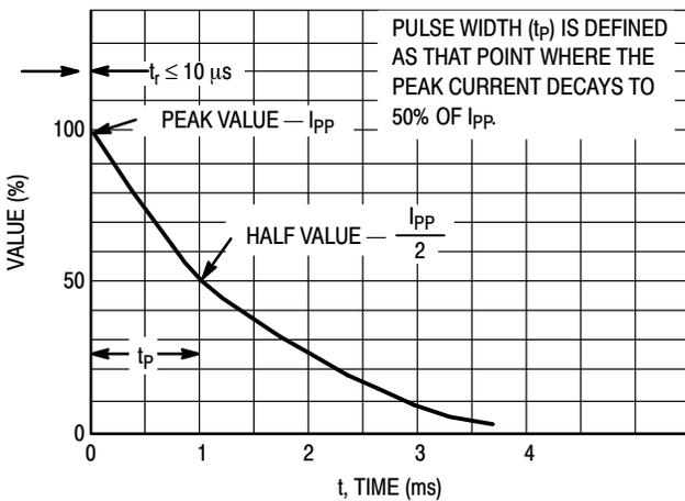
Figure 5. Pulse Waveform
