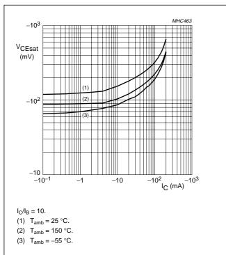
Fig.6 Collector-emitter saturation voltage as a function of collector current.
