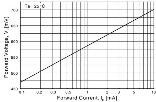
Figure 4. Forward Voltage vs Forward Current
