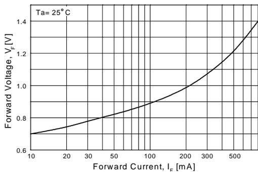
Figure 5. Forward Voltage vs Forward Current
