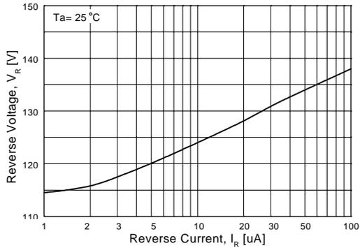
Figure 1. Reverse Voltage vs Reverse Current
