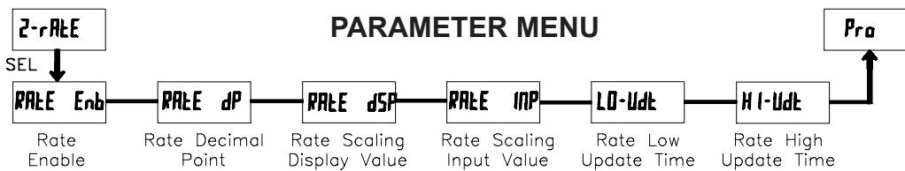
Module 2 is the programming for the rate parameters. For maximum input frequency, Rate Enable should be set to NO when not in use. When set to NO, the remaining rate parameters are not accessible. The rate value is shown with an annunciator of “P” in the Display Mode.
