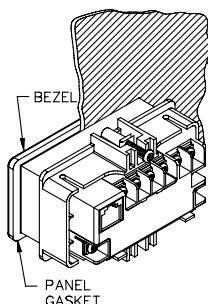
While holding the unit in place, push the panel latch over the rear of the unit so that the tabs of the panel latch engage in the slots on the case. The panel latch should be engaged in the farthest forward slot possible. To achieve a proper seal, tighten the latch screws evenly until the unit is snug in the panel (Torque to approx. 28 to 36 in-oz [0.202 to 0.26 N-m]). Do not over-tighten the screws.
