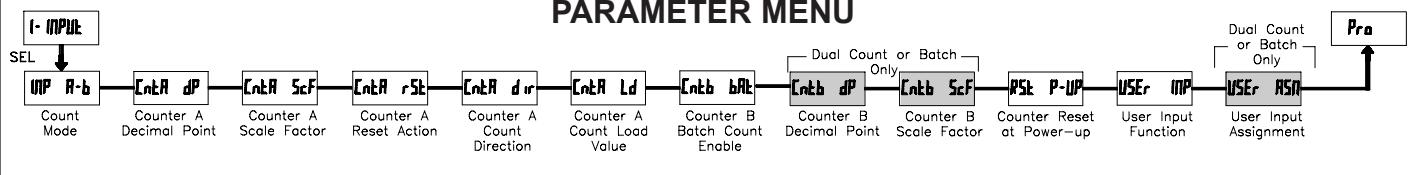
Shaded area selections only apply when Counter B is enabled (Dual Counter mode or batch counter).
