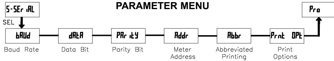
The Serial Communications Parameters are only accessible when an optional RS232 or RS485 serial communications module is installed in the meter.
