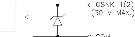
Note: Output Common is not isolated from DC Power Common. Load must be wired between OSNK terminal and V+ of the load supply.
