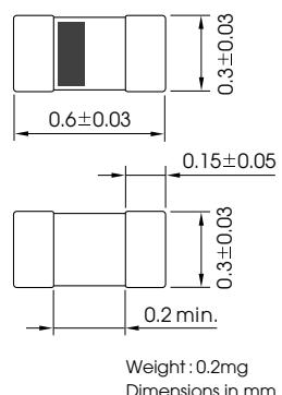
The 0603 type allows reduction of the dimension by 64% (68%, if implementation area, including the land pattern, is considered), and of the volume by 78% compared to the 1005 type.
