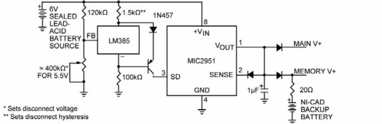
For values shown, Regulator shuts down when  $V_{IN} < 5.5\text{ V}$  and turns on again at  $6.0\text{ V}$ . Current drain in disconnected mode is  $150\mu\text{A}$ .
