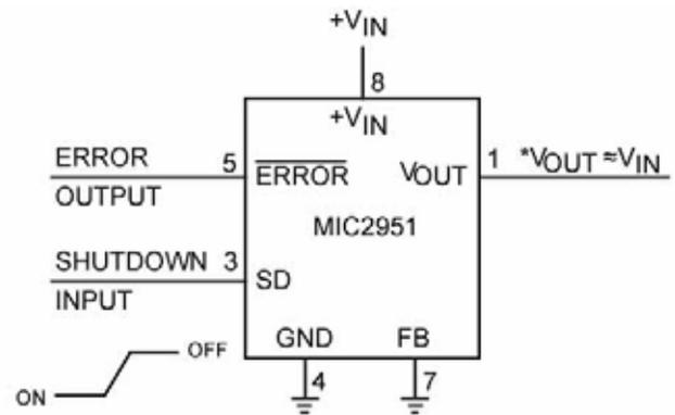
\*MINIMUM INPUT-OUTPUT VOLTAGE RANGES FROM 40mV TO 400mV, DEPENDING ON LOAD CURRENT. CURRENT LIMIT IS TYPICALLY 160mA.
