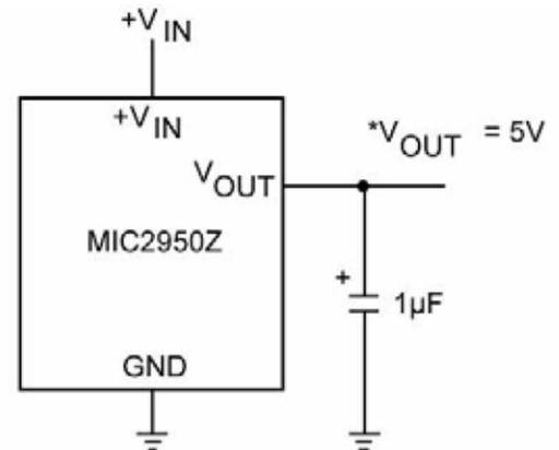
\* MINIMUM INPUT-OUTPUT VOLTAGE RANGES FROM 40mV TO 400mV, DEPENDING ON LOAD CURRENT.
