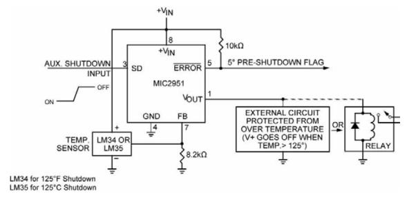
**System Over Temperature Protection Circuit**
