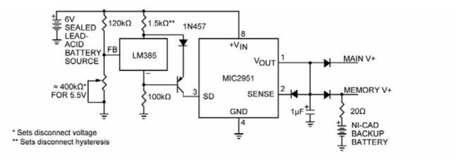
For values shown, Regulator shuts down when V<sub>IN</sub> < 5.5 V and turns on again at 6.0 V. Current drain in disconnected mode is 150μA.
