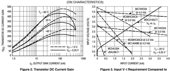
Figure 3. Input V–I Requirement Compared to Possible Source Logic Outputs
