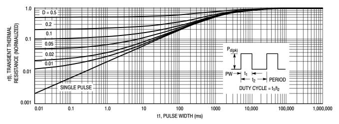
Figure 12. Transient Thermal Response for MDC3105LT1
