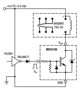
Figure 14. A 140 mW, 5.0 V Relay with TTL Interface
