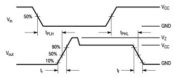
Figure 1. Switching Waveforms
