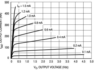
Figure 5. Transistor Output V-I Characteristic
