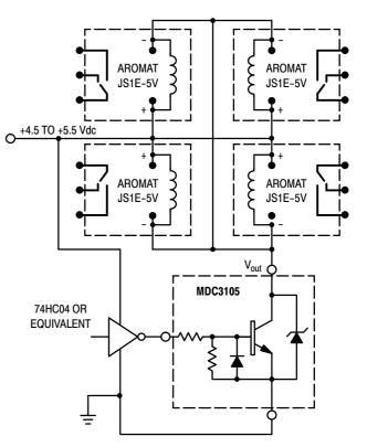
Figure 15. A Quad 5.0 V, 360 mW Coil Relay Bank
