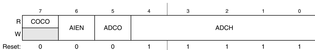
Figure 10-3. Status and Control Register (ADCSC1)
