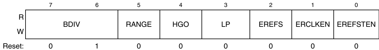
Figure 11-4. ICS Control Register 2 (ICSC2)
