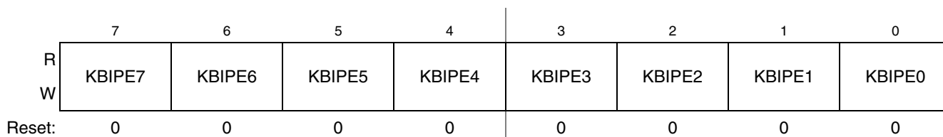
Figure 7-4. KBI Interrupt Pin Select Register (KBIPE)
