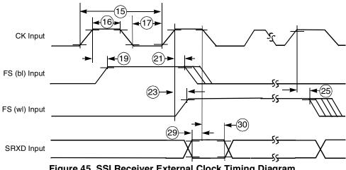
Figure 45. SSI Receiver External Clock Timing Diagram
