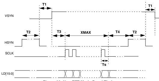
Figure 22. Non-TFT Mode Panel Timing
