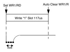
Figure 48. Write 1 Timing
