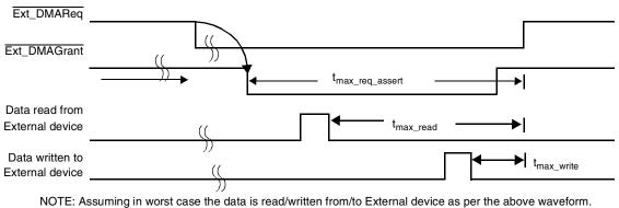
Figure 5. Safe Maximum Timings for External Request De-Assertion
