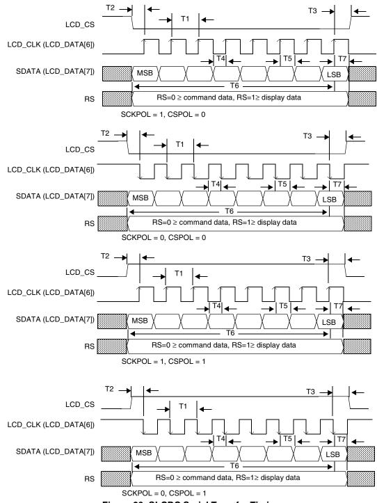
Figure 23. SLCDC Serial Transfer Timing
