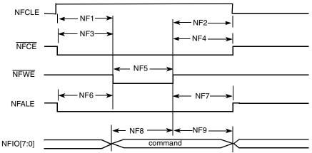
Figure 33. Command Latch Cycle Timing Dlagram
