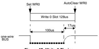
Figure 47. Write 0 Timing
