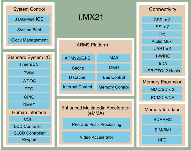
Figure 1. i.MX21 Functional Block Diagram
