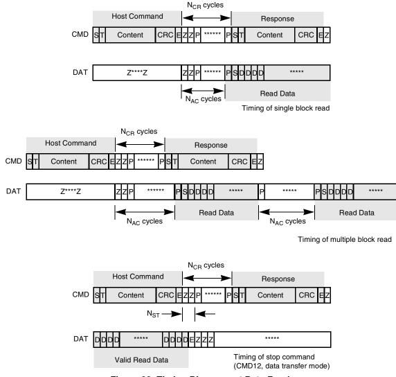
Figure 28. Timing Diagrams at Data Read
