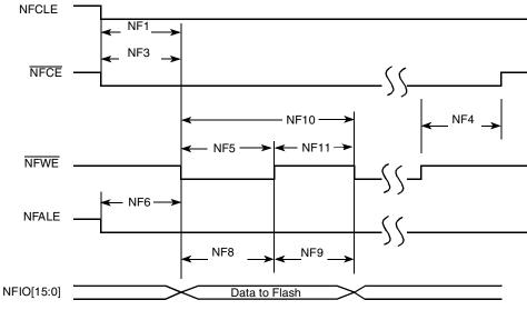
Figure 35. Write Data Latch Timing Dlagram
