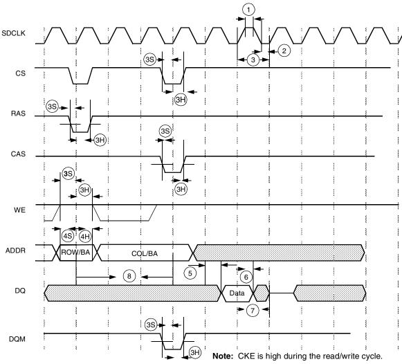
Figure 38. SDRAM Read Cycle Timing Diagram
