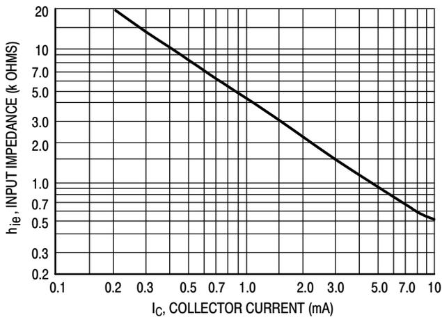
Figure 11. Input Impedance
