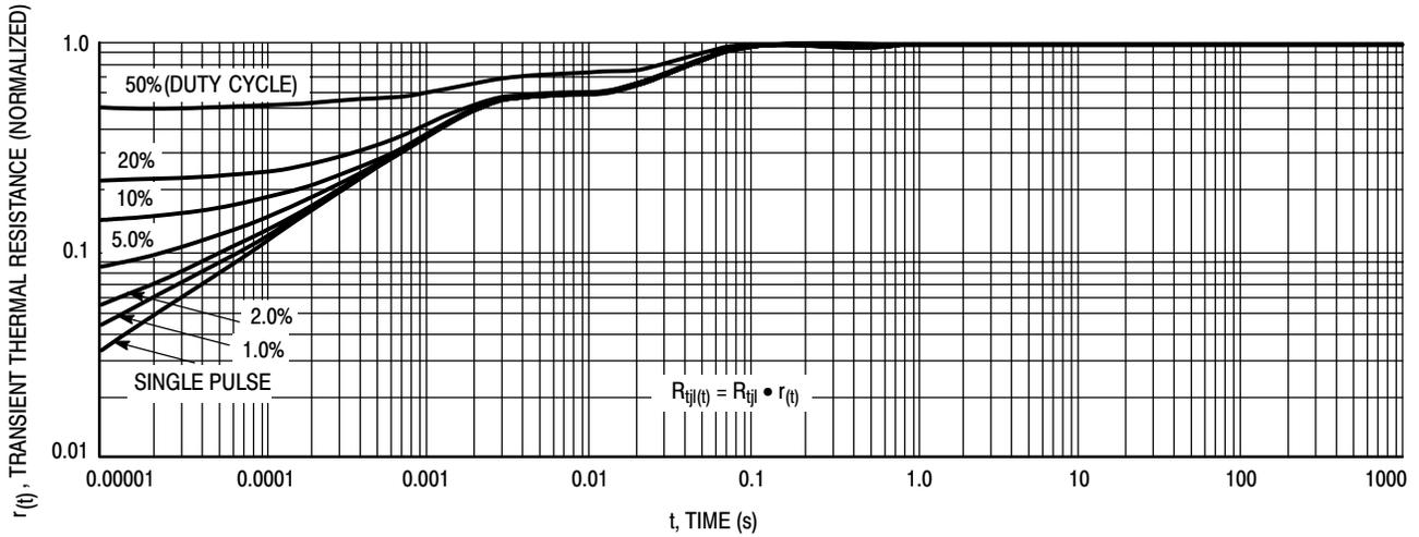
Figure 9. Thermal Response Junction to Case (Per Leg)
