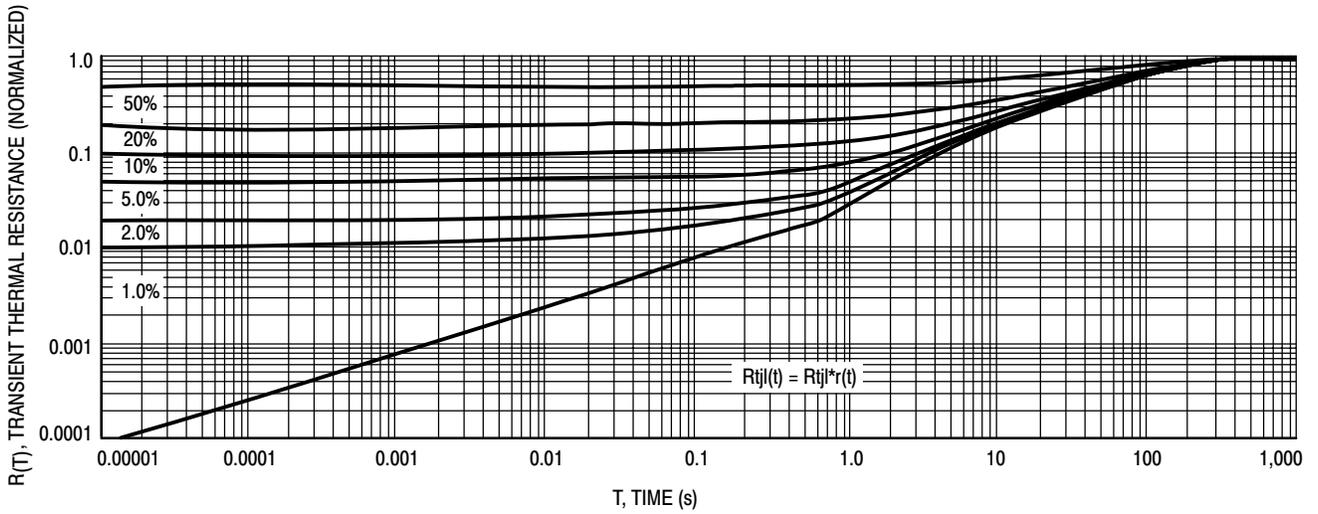
Figure 10. Thermal Response Junction to Ambient (Per Leg)
