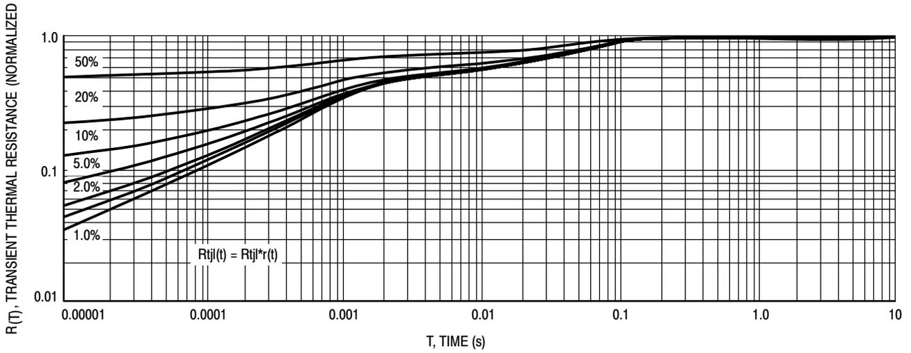
Figure 9. Thermal Response Junction to Lead (Per Leg)
