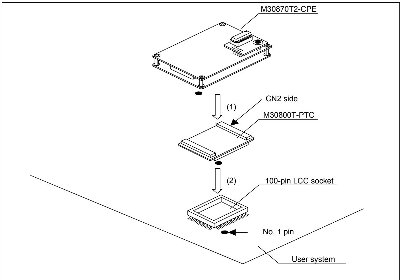
Figure 2.12 Connecting to a 100-pin LCC socket
