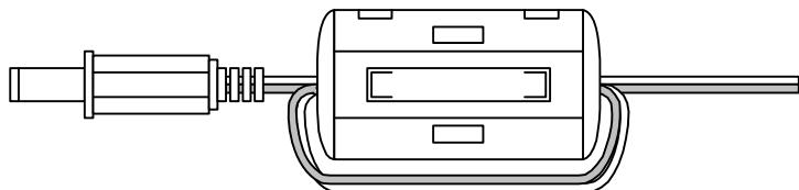
Figure 2.2 Attaching the ferrite core
