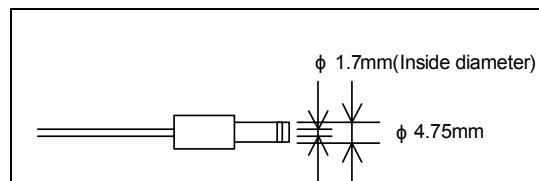
Figure 2.4 Applicable plug specifications
