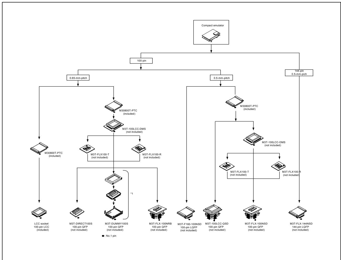
Figure 2.11 Connection of the M30870T2-CPE and user system
