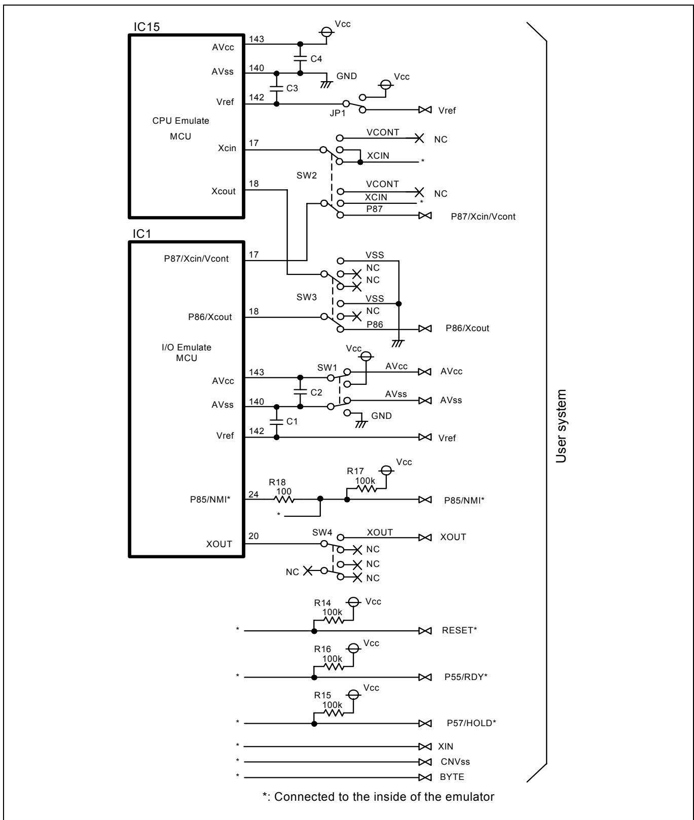
Figure 4.1 Connection diagram (when using M30870T-EPBM REV.B) (1/3)
