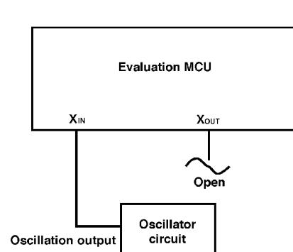
Figure 2.25 External oscillator circuit
