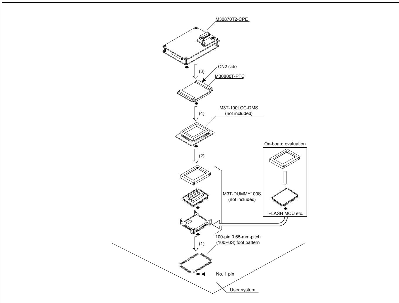
Figure 2.13 Connecting to a 100-pin 0.65-mm-pitch foot pattern (part 1)
