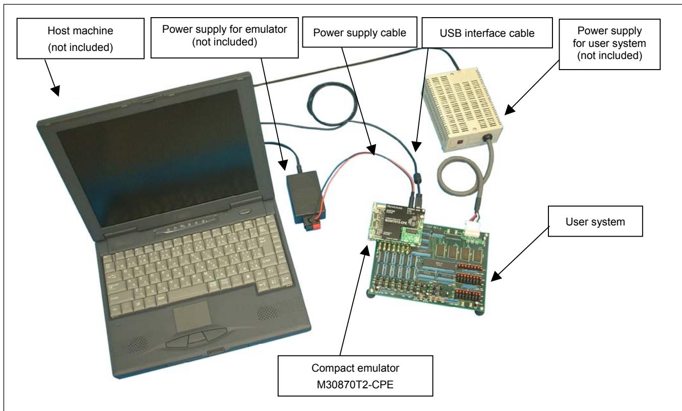
Figure 1.1 System configuration
