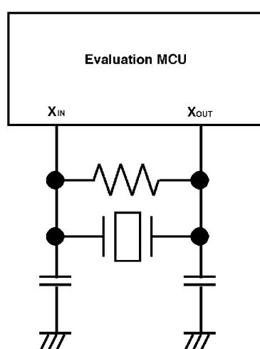
Figure 2.26 Circuit in which oscillation does not occur
