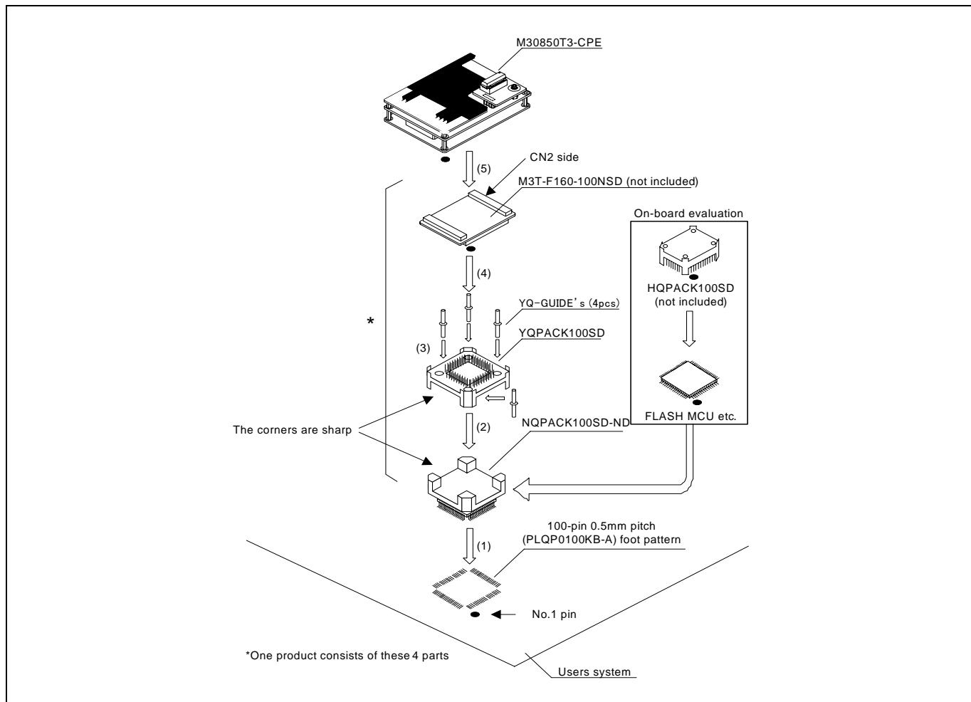
Figure 2.16 Connecting to a 100-pin 0.5mm pitch foot pattern
