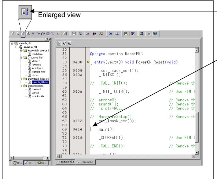
Setup procedure for running the program up to the cursor position
