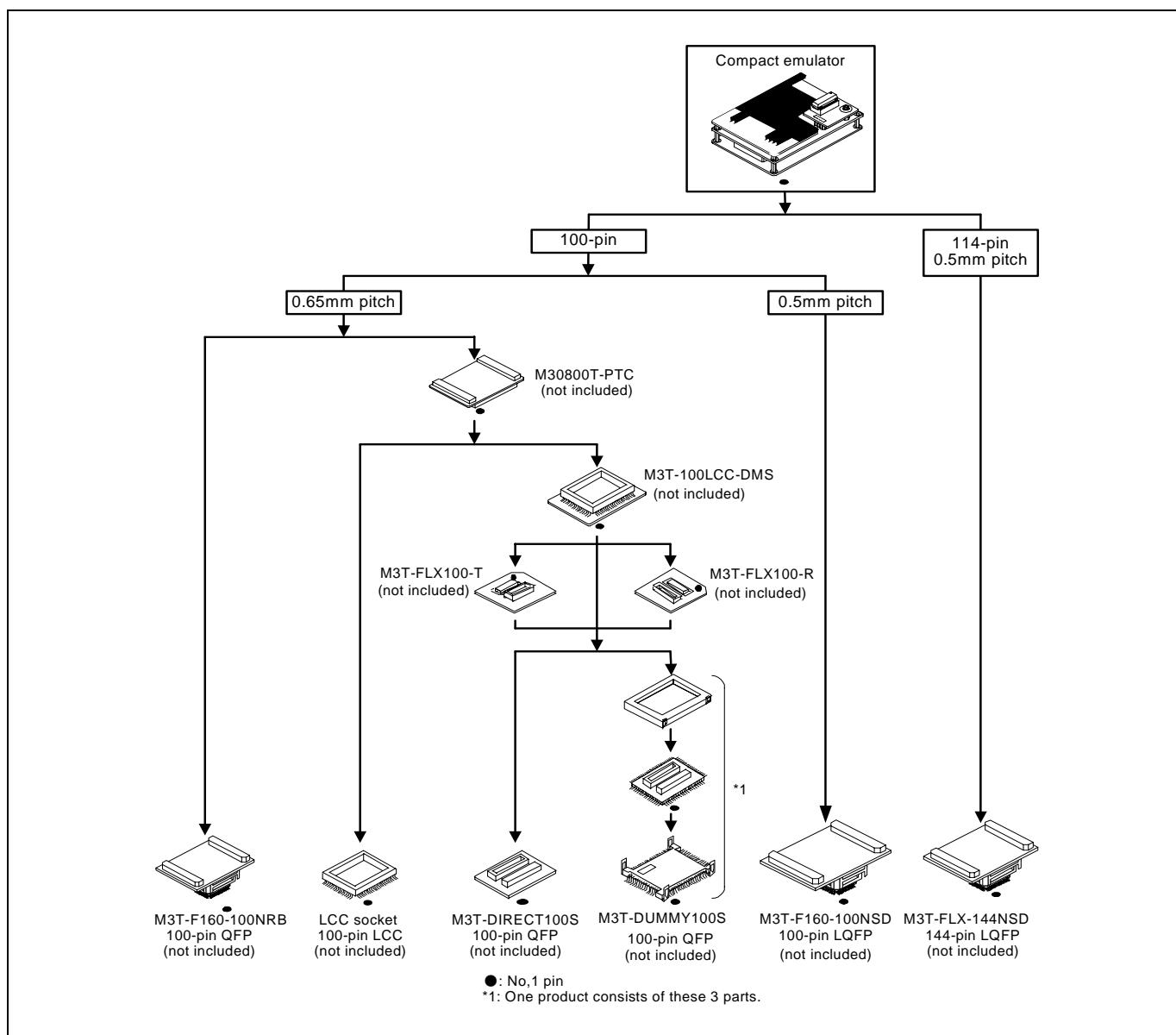
Figure 2.11 Connection of the M30850T3-CPE and user system
