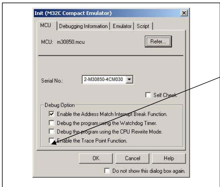
Using or not using the trace point function
