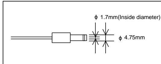
Figure 2.4 Applicable plug specifications
