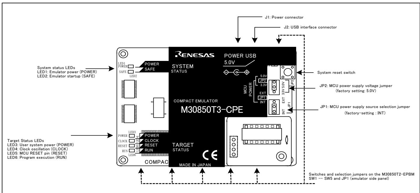
Figure 1.2 Names of the LEDs on the upper panel of the M30850T3-CPE
