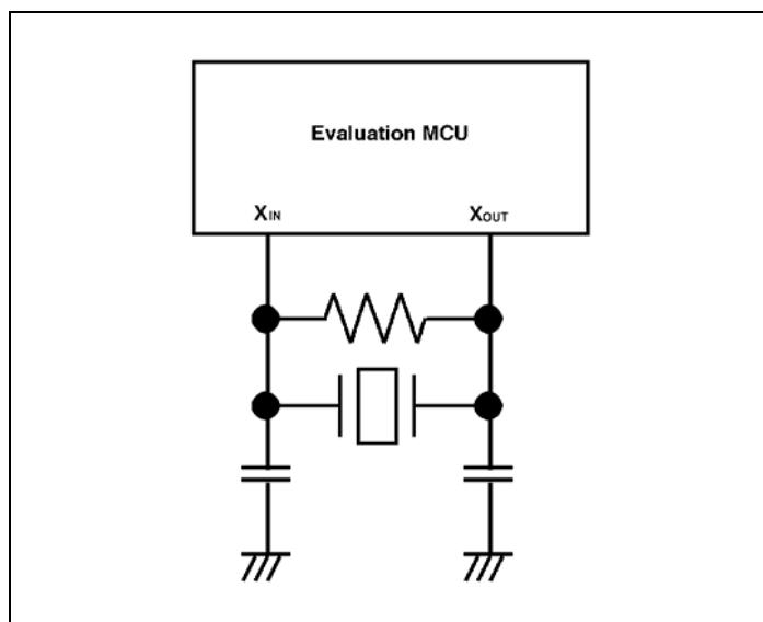
Figure 2.23 Circuit in which oscillation does not occur
