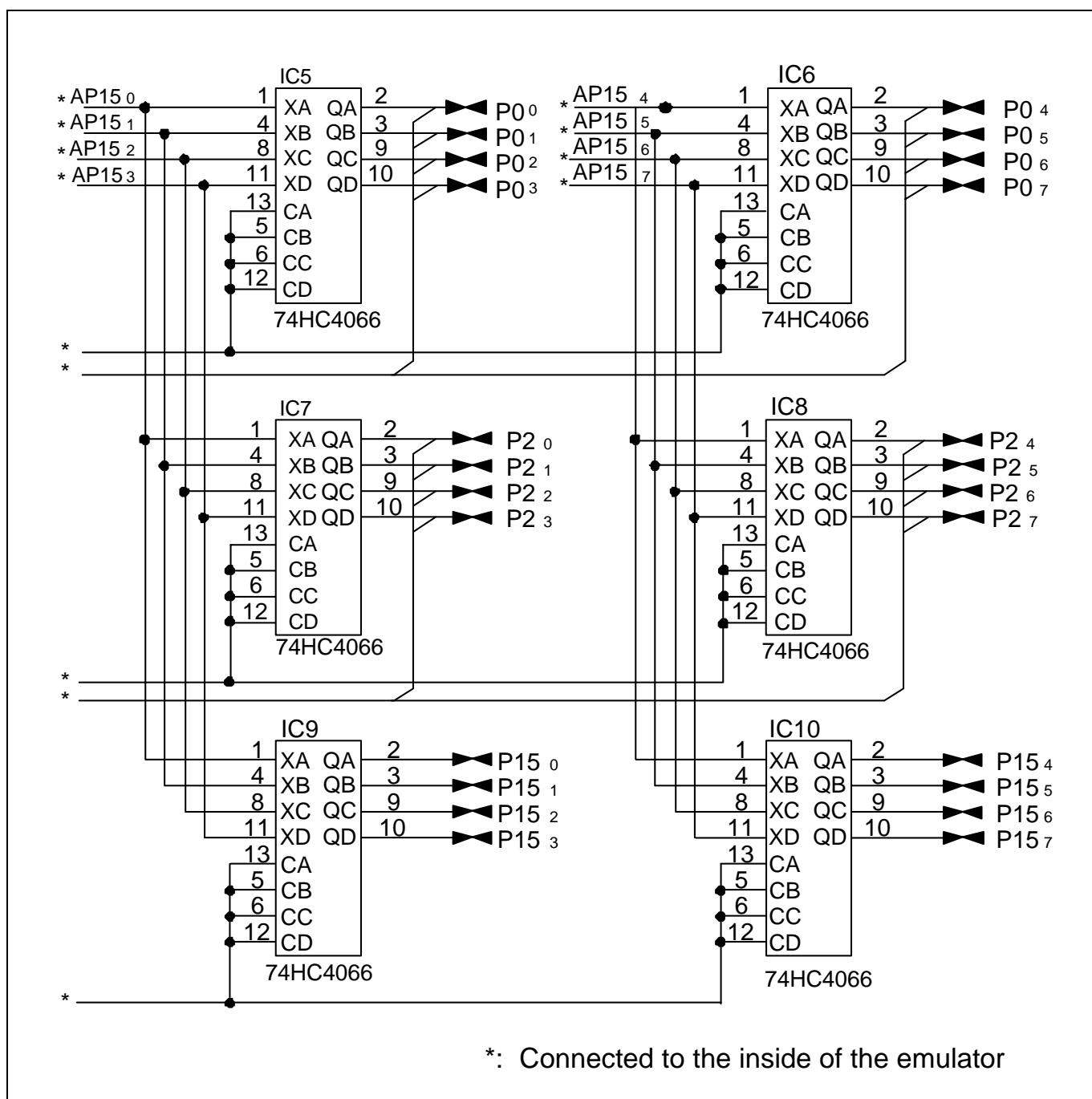
Figure 4.7 Connection diagram (2/2)
