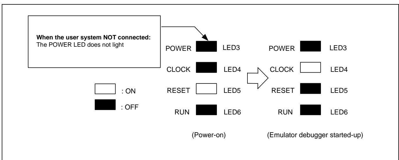
Figure 2.8 Target status LEDs display when the emulator starts up normally (when user system not connected)
