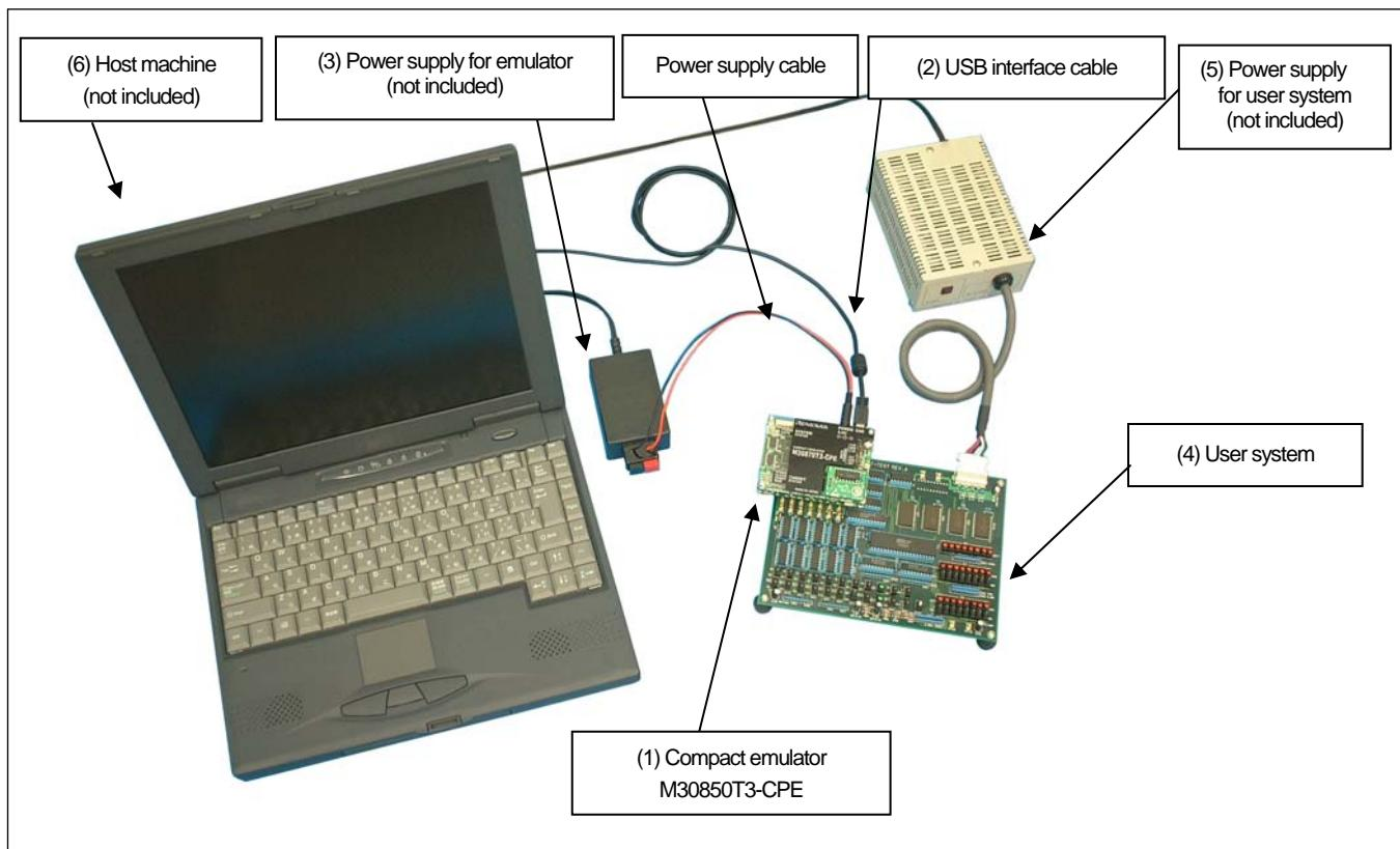
Figure 1.1 System configuration
