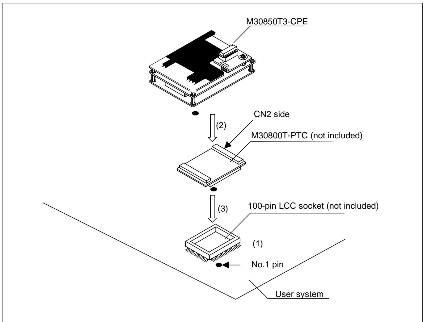
Figure 2.12 Connecting to a 100-pin LCC socket
