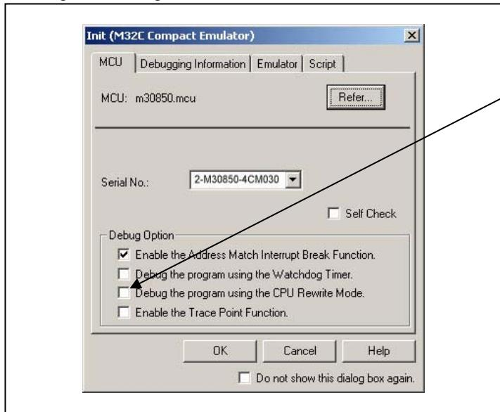
Using or not using CPU rewrite mode
