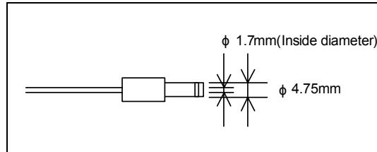
Figure 2.4 Applicable plug specifications
