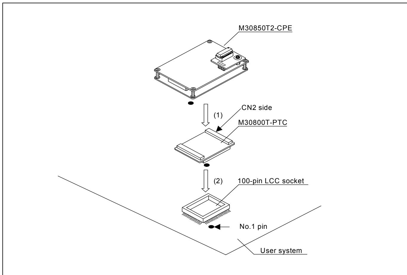
Figure 2.12 Connecting to a 100-pin LCC socket
