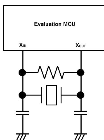
Figure 2.25 Circuit in which oscillation does not occur
