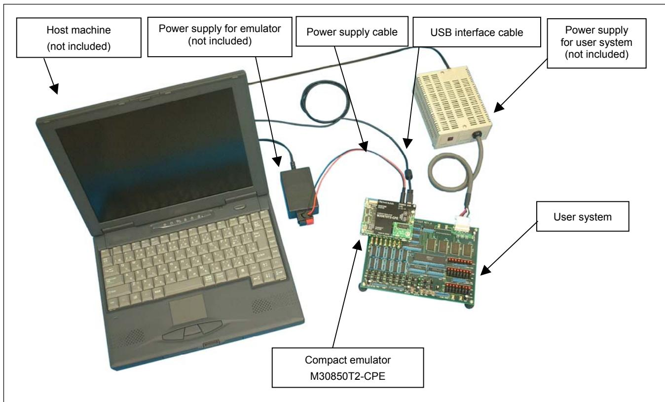
Figure 1.1 System configuration
