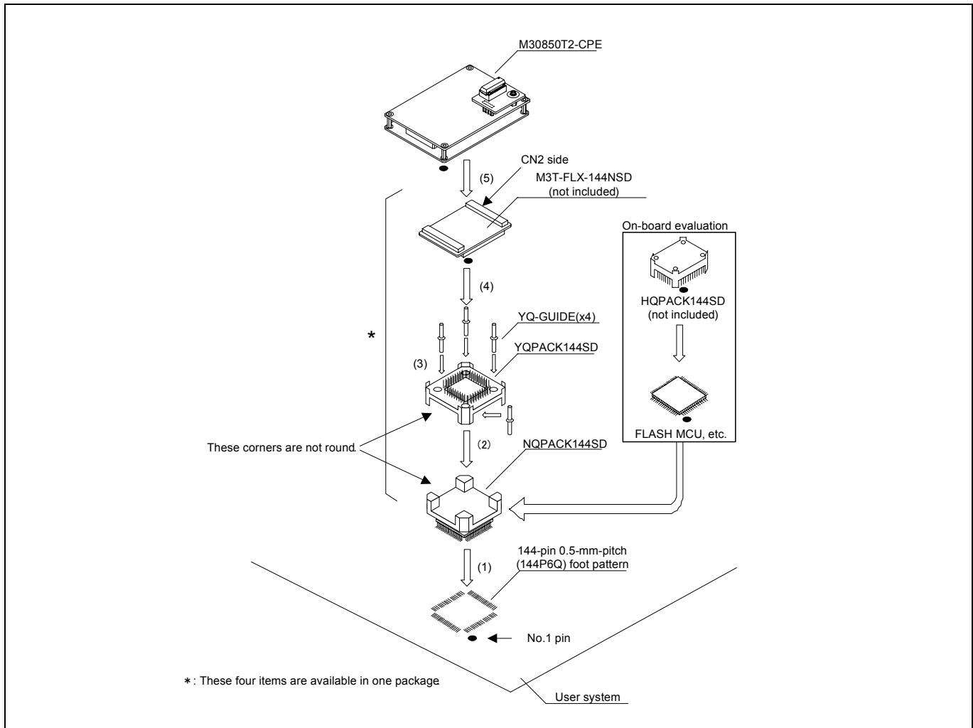
Figure 2.19 Connecting to a 144-pin 0.5-mm-pitch foot pattern
