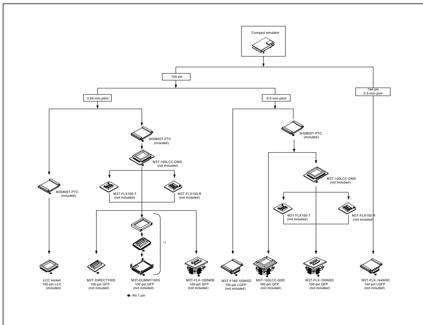
Figure 2.11 Connection of the M30850T2-CPE and user system
