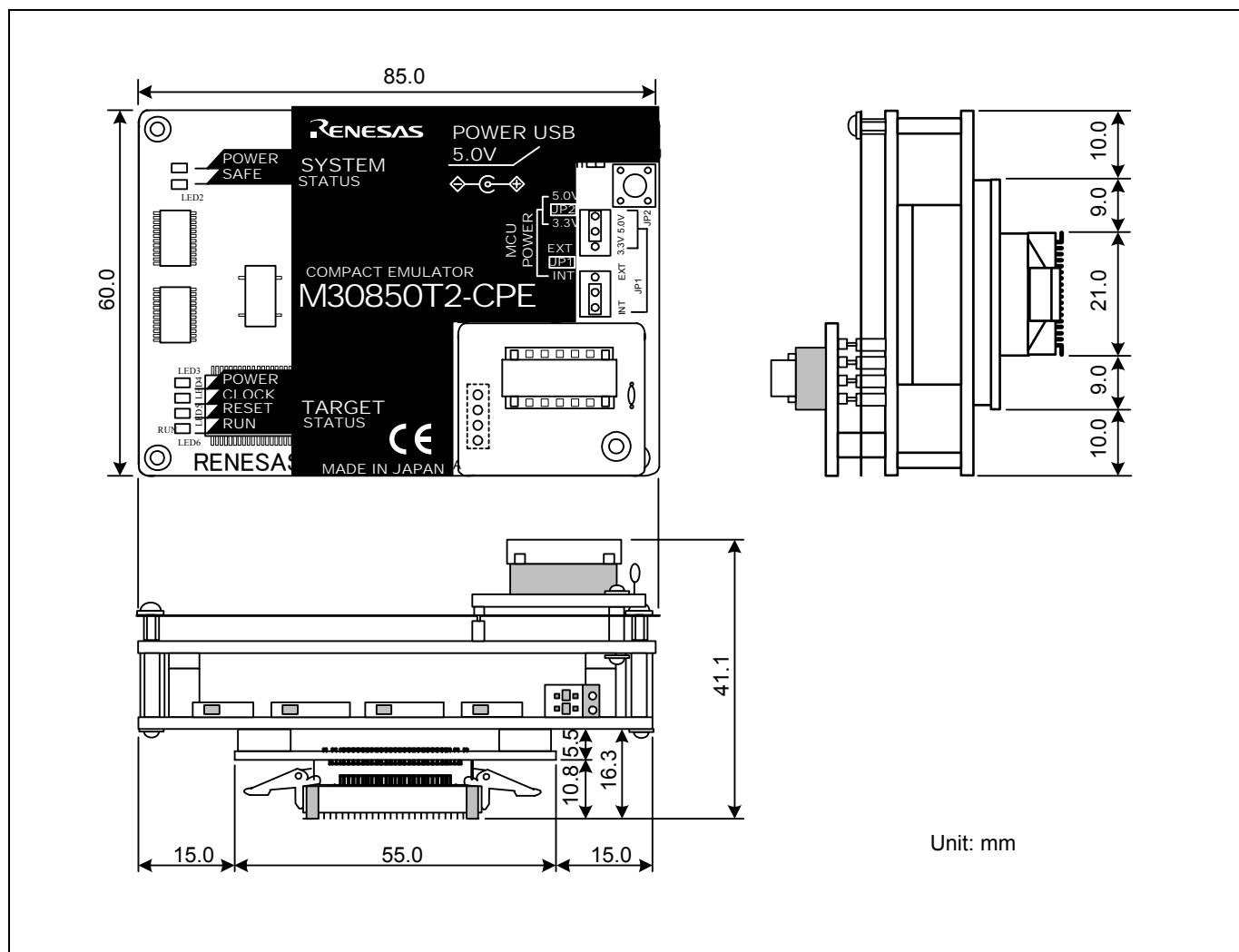
Figure 4.3 External dimensions of the compact emulator
