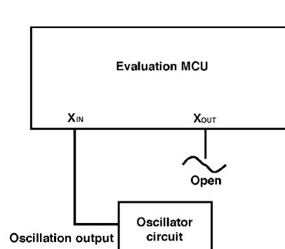
Figure 2.24 External oscillator circuit
