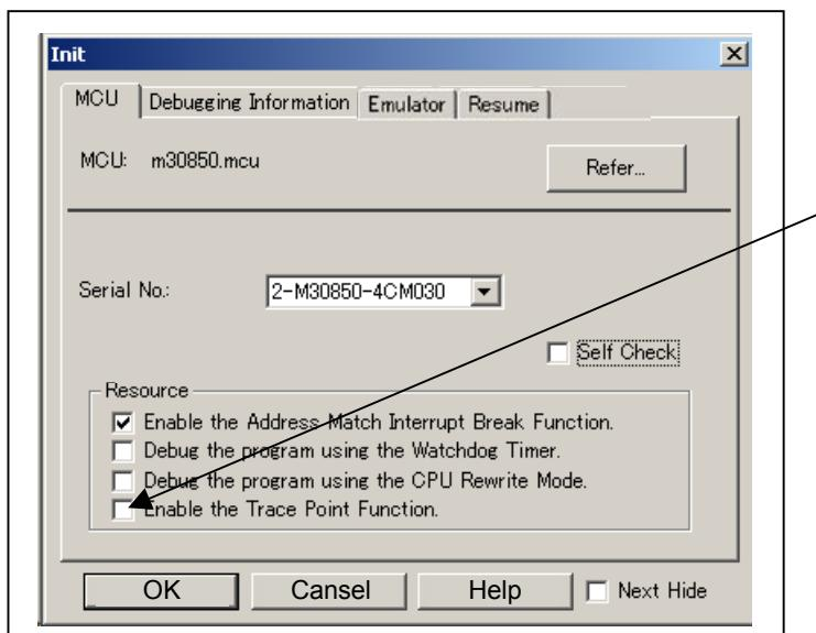
Using or not using the trace point function
