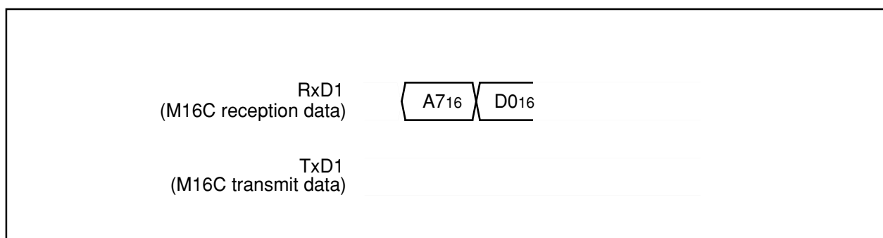
Figure 1.32.27. Timing for erasing all unlocked blocks
