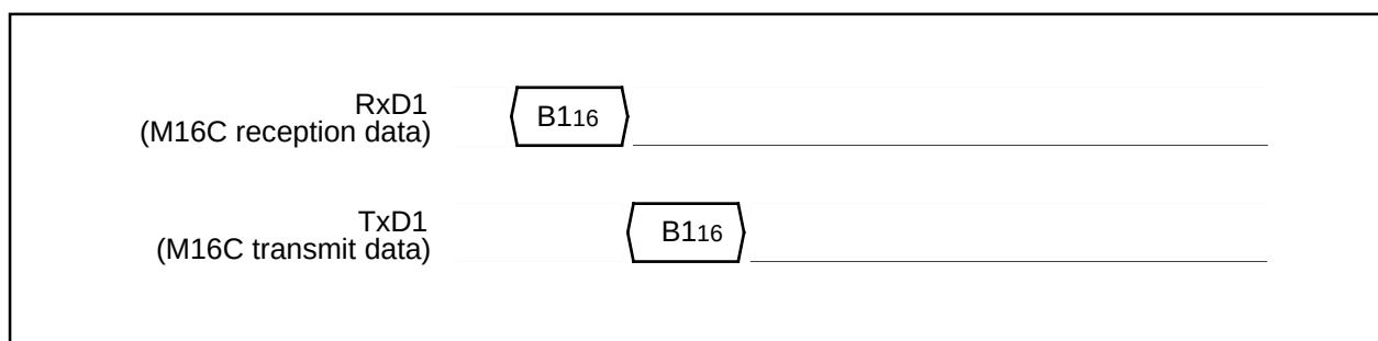
Figure 1.29.40. Timing of baud rate 19200
