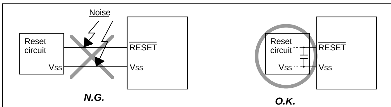
Figure 1.1.2. Wiring for RESET pin
