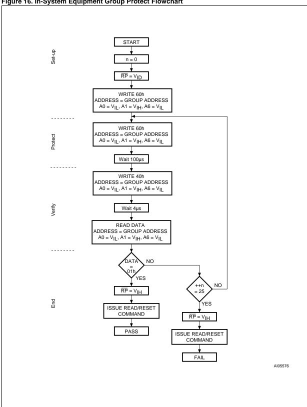
Figure 16. In-System Equipment Group Protect Flowchart
