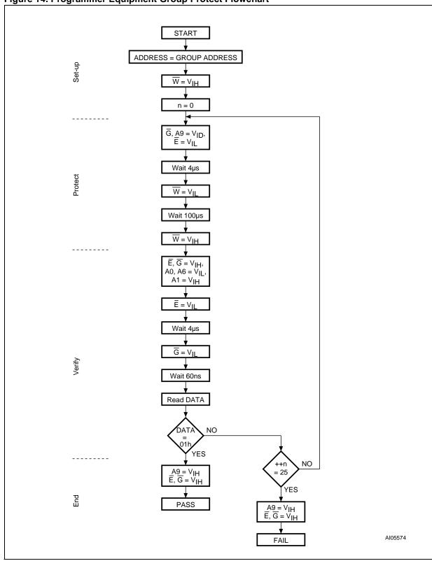
Figure 14. Programmer Equipment Group Protect Flowchart
