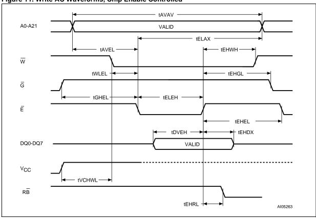
Figure 11. Write AC Waveforms, Chip Enable Controlled
