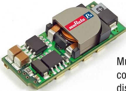
Murata Power Solutions' miniature POL switching DC/DC converters are ideal regulation and supply elements for distributed power and intermediate bus architectures.
