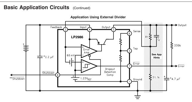
\* Minimum capacitance shown to assure stability, but may be increased without limit. Larger output capacitor provides improved dynamic response.
