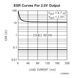
**IMPORTANT:** The output capacitor must maintain its ESR in the stable region *over the full operating temperature range of the application* to assure stability.
