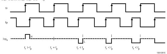
Note 15: fr is phase detector input from reference counter. fp is phase detector input from programmable N counter. Phase difference detection range: -  $2\pi$  to +  $2p\pi$ .
