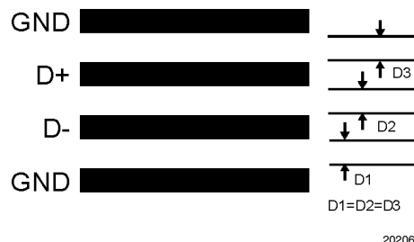
FIGURE 9. Ideal Diode Trace Layout
