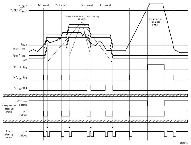
Note: Event Interrupt mode is drawn as if the user is reading the part. If the user doesn't read, the outputs would go low and stay that way until the LM76 is read.
