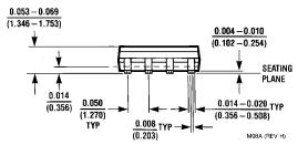
8-Lead (0.150" Wide) Molded Small Outline Package (SOP), JEDEC Order Number LM76CNM-3, LM76CNMX-3, LM76CHM-5 or LM76CHM-5X **NS Package Number M08A**
