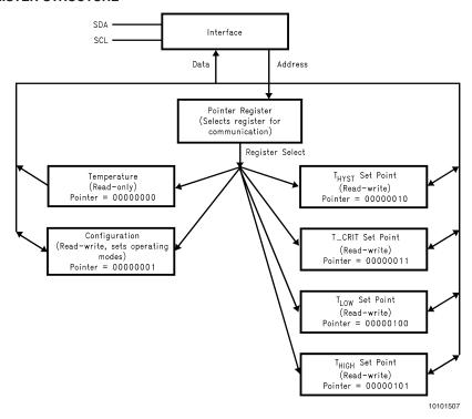
There are four data registers in the LM76, selected by the Pointer register. At power-up the Pointer is set to "00"; the location for the Temperature Register. The Pointer register latches the last location it was set to. In Interrupt Mode, a read from the LM76 resets the INT output. Placing the device in Shutdown mode resets the INT and T\_CRIT\_A outputs. All registers are read and write, except the Temperature register which is read only.
