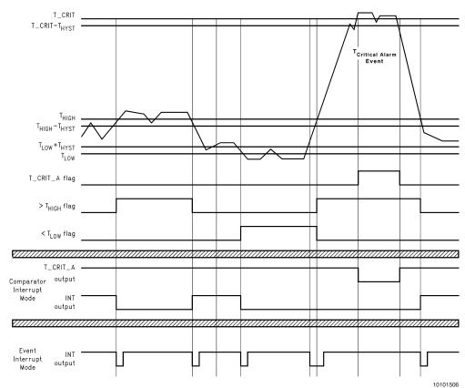
Note: Event Interrupt mode is drawn as if the user is reading the part. If the user doesn't read, the outputs would go low and stay that way until the LM76 is read.
