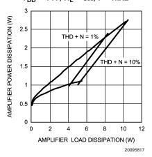
**Amplifier Power Dissipation** vs Total Load Power Dissipation  $V_{DD} = 9V, R_L = 8\Omega, f = 1kHz$
