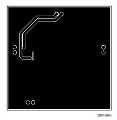
FIGURE 4. Recommended SD PCB Layout Bottom Layer
