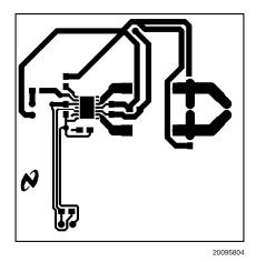
FIGURE 3. Recommended SD PCB Layout Top Layer
