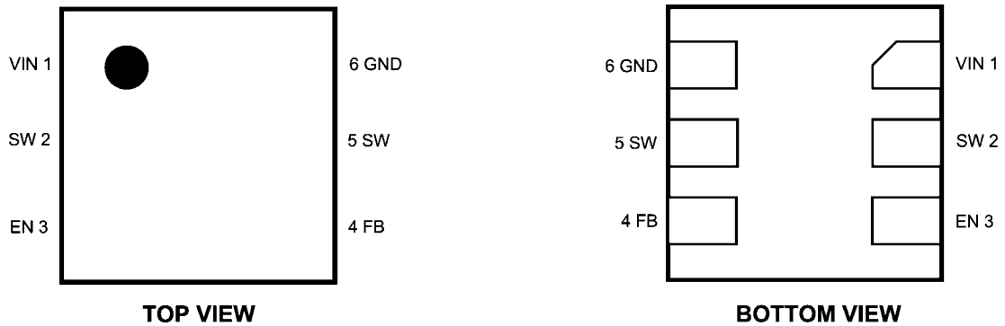
FIGURE 4. 6 Pin LLP Package
