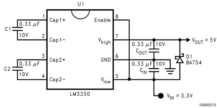
FIGURE 2. Step-Up Converter
