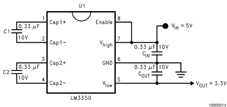
FIGURE 3. Step-Down Converter
