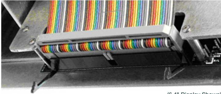
Figure 3.5 – Connect Ribbon Cable to the Display Kit
