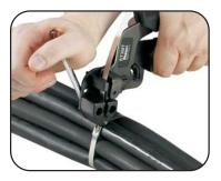
3. Maintain tension and rotate cut-off handle
