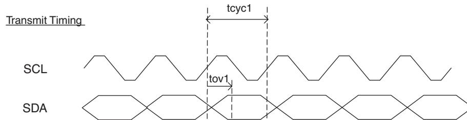
Figure 13. EEPROM Interface Output Transmit Timing Diagram
