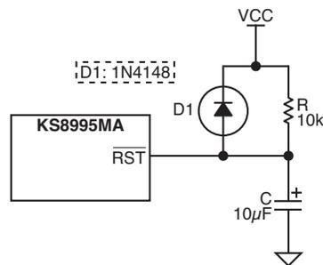
Figure 24. Recommended Circuit for Interfacing with CPU/FPGA Reset
