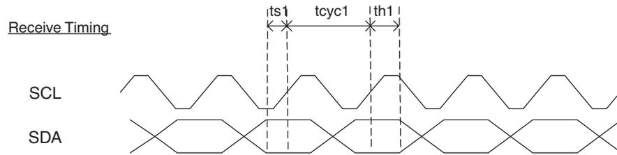
Figure 12. EEPROM Interface Input Receive Timing Diagram
