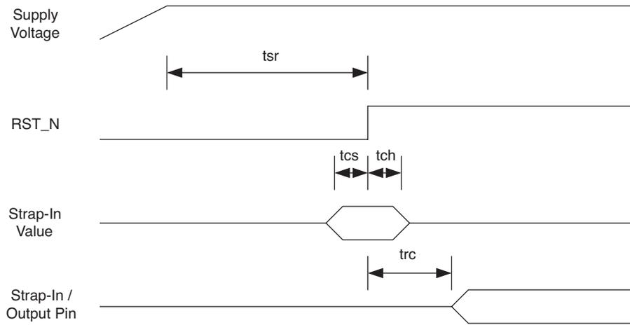
Figure 22. Reset Timing
