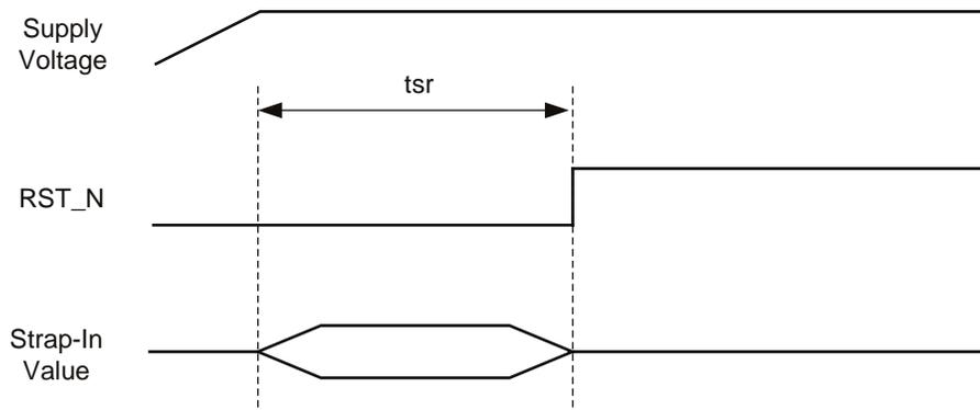
Figure 9. Reset Timing
