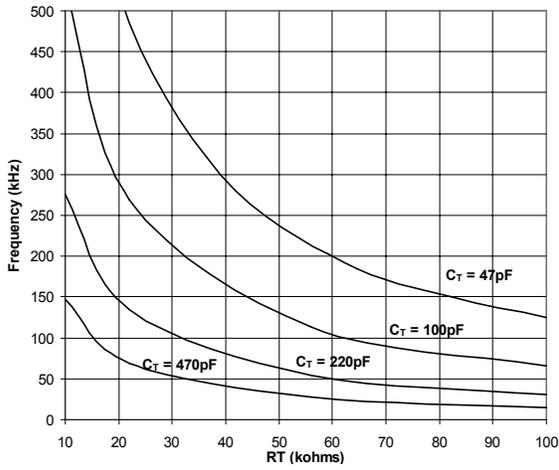
Fig. 1 Typical Output Frequency (-25°C to 125°C)
